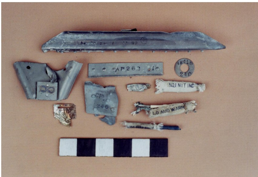
Some of the many pieces Peter recovered from an A-12 crash site in Utah that was also cleaned up with an effort to retrieve every scrap of material from the craft. Notice the inspection markings and serial numbers that can trace the debris back to the skunkworks.
