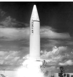
A Jupiter missile's boost phase lasted about 158 seconds and the vernier engines cutoff around 174 seconds. This all happened between 80 and 120 miles altitude. For a distance of 140 miles, the angle of elevation would be between 30 and 40 degrees.
